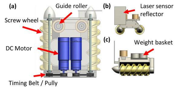
FIGURE 1. Modeling of a screw-based crawling robot.
