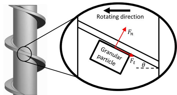
FIGURE 2. Forces between the blade of the wheel and the ground particle on the granular surface ( $F_n$ : normal force,  $F_t$ : tangent force,  $\theta$ : angle of blade).
