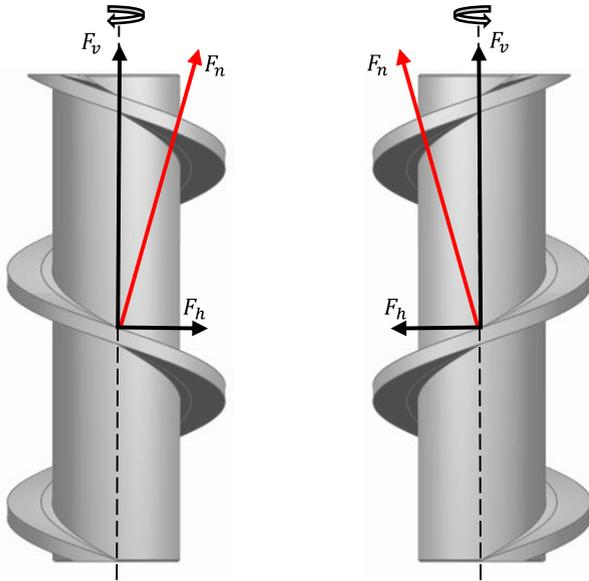
**FIGURE 3.** Forces of two screw wheels rotating in opposite directions ( $F_n$ : normal force,  $F_v$ : vertical force,  $F_h$ : horizontal force. The relation equation between them is as follows:  $F_v = F_n \times \cos\theta$ ,  $F_h = F_n \times \sin\theta$  ( $\theta$  is from Fig.2)).
