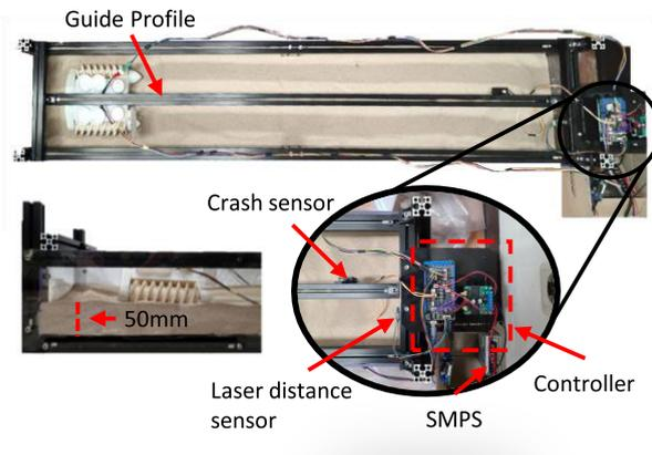
**FIGURE 4.** Structure of test bench.
