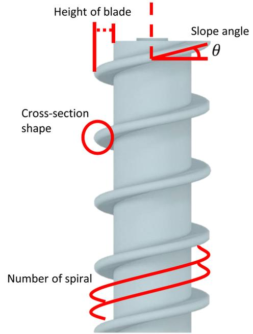
**FIGURE 5.** Design parameters of screw wheel.
