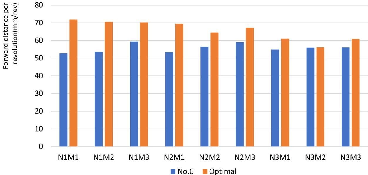
**FIGURE 9.** Comparison of forward distance per revolution between No. 6 and optimized design (User condition: Load (g) (N1 = 0, N2 = 500, N3 = 1,000); Motor rpm (rev/min) (M1 = 250, M2 = 300, M3 = 350)).
